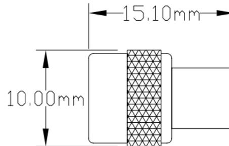
Coaxial fixed terminations absorb RF & microwave energy and are commonly used as dummy loads of antenna and transmitter. They are also used as match ports in many multiport microwave devices such as circulator and directional coupler to make these ports which are not involved in the measurement be terminated in their characteristic impedance in order to ensure an accurate measurement.
