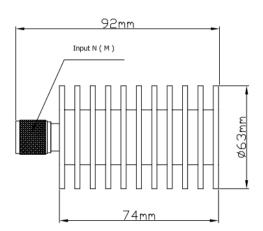
Coaxial fixed terminations absorb RF& microwave energy and are commonly used as dummy loads of antenna and transmitter. They are also used as match ports in many multiport microwave devices such as circulator and directional coupler to make these ports which are not involved in the measurement be terminated in their characteristic impedance in order to ensure an accurate measurement.
