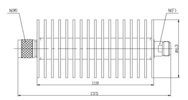
Coaxial fixed attenuators are used in absorbing energy of transmission line, expanding power range and controlling power level, they are also used in accurately measuring power or spectrum of RF microwave transmitters accompany with small power meter, comprehensive tester or spectrum analyzer.
